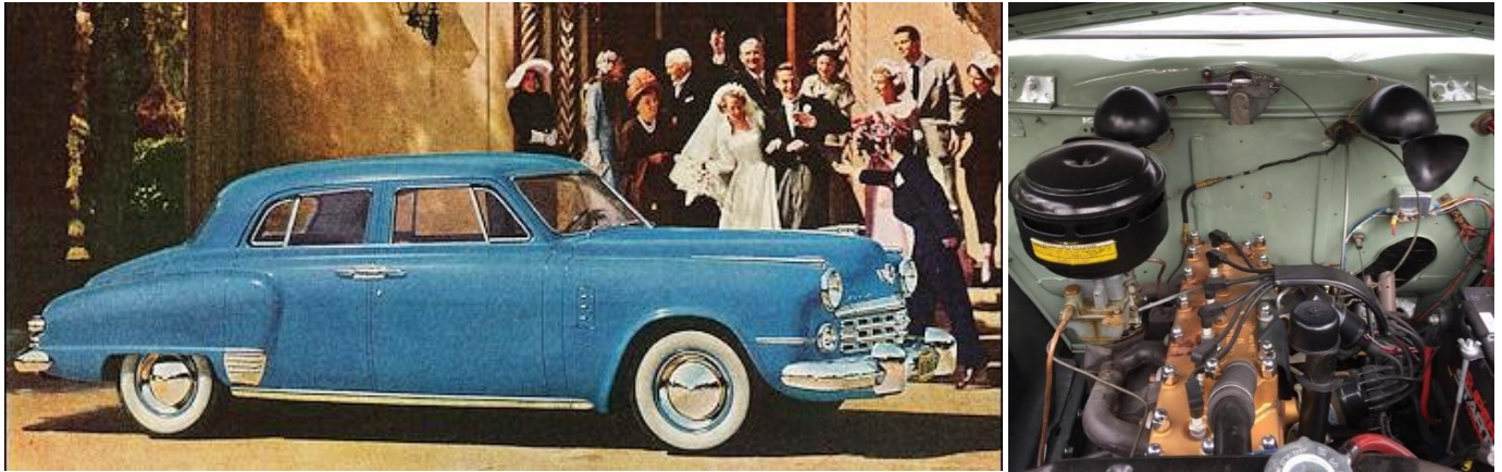
Above left a 1949 Studebaker Land Cruiser. Above right a L-head straight six-cylinder engine
