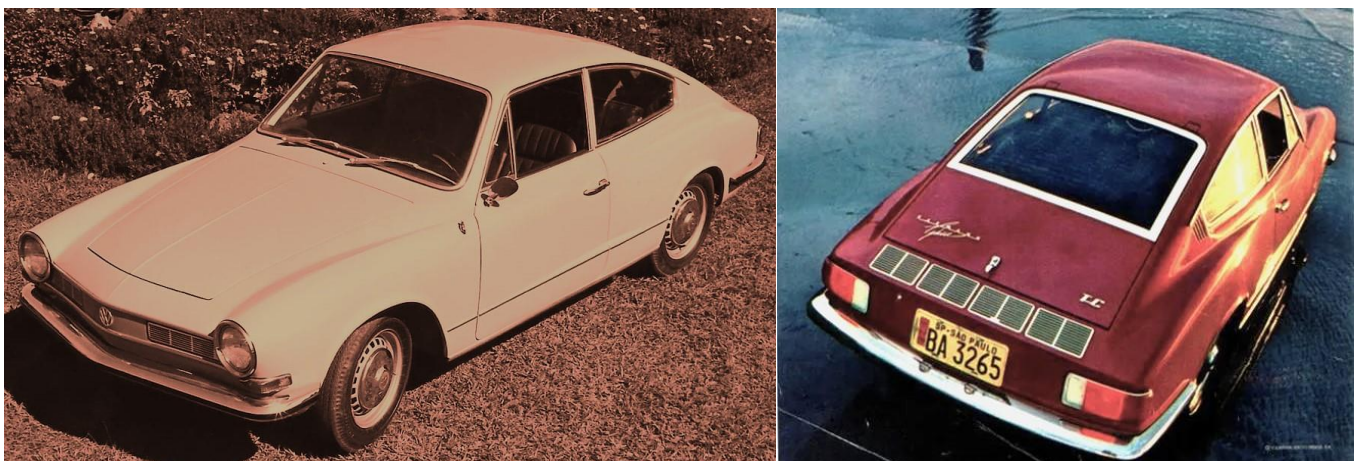
Factory pics of the Karmann Ghia TC (Type 145) and note the large single piece tailgate over the rear engine bay.
