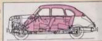
The short horizontally-opposed engine was mounted well forward, increasing the car's interior space.
