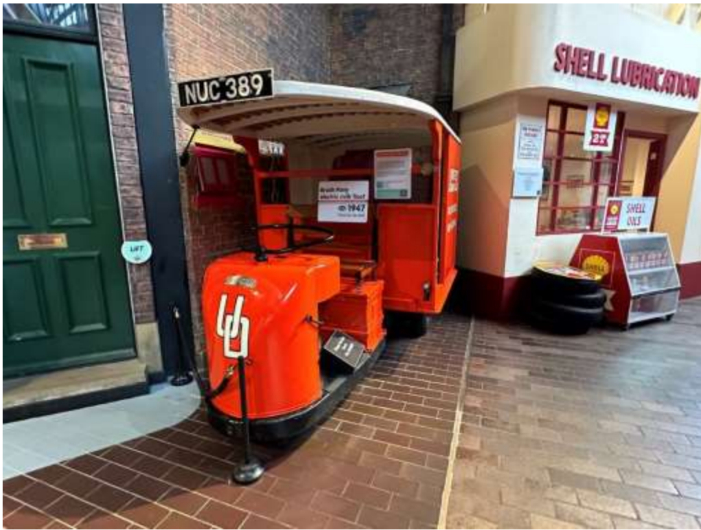
Typical battery electric “milk float”—home-delivered dairy products were delivered with electric vehicles so as not to wake up sleeping residents.
