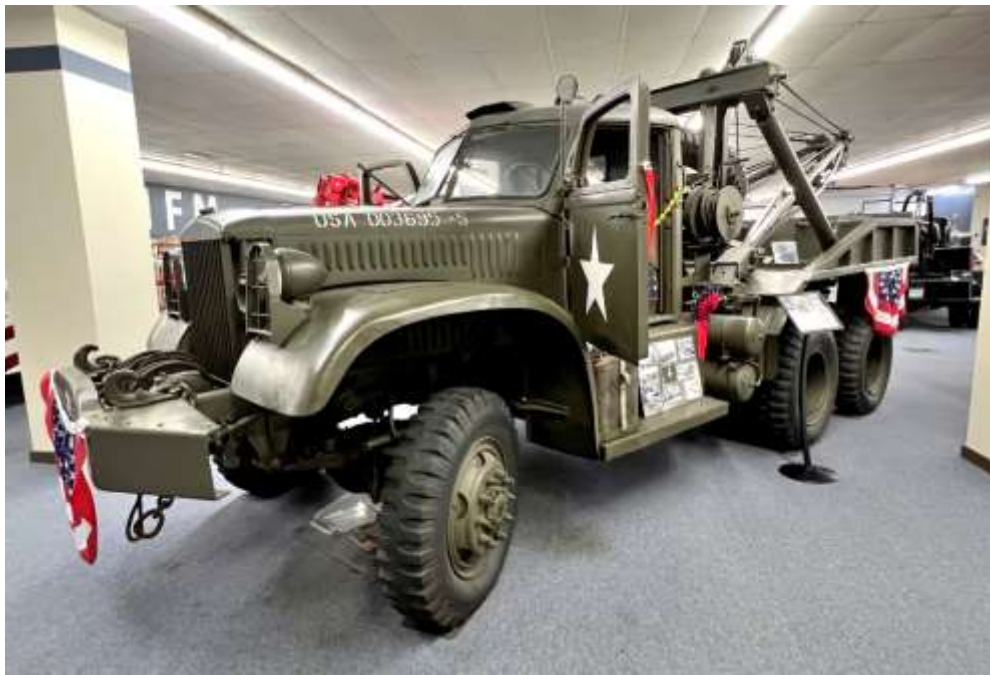
13) 1943 Diamond T 969 truck with Holmes W-45 wrecker. Holmes made the W-45 from 1941 to 1949, manufacturing more than 7000 units. This wrecker was one of many used along the U.S. Army's Red Ball Express supply routes in France and Belgium.
