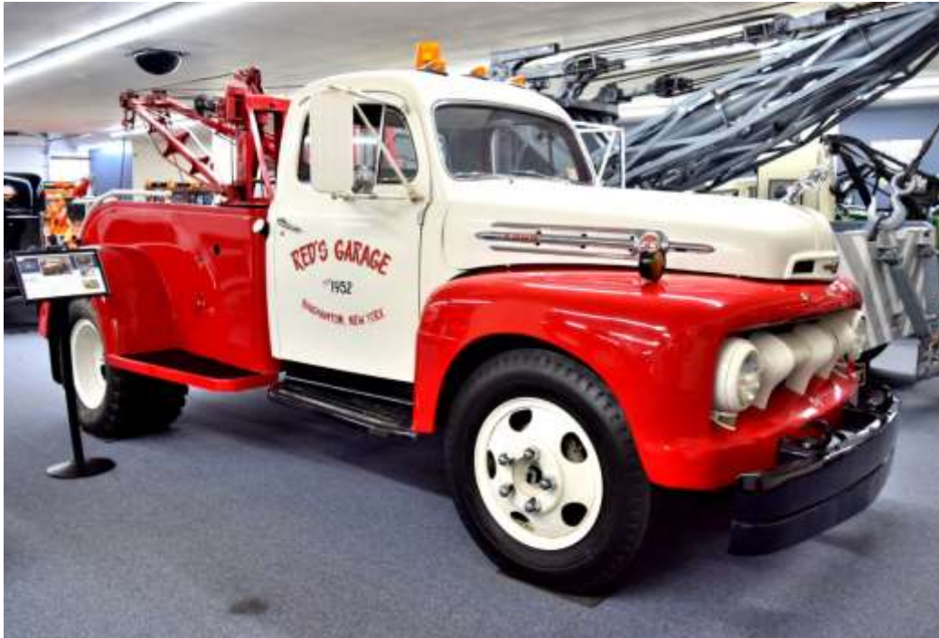
21) 1952 Ford F-6 truck with Holmes 460 "Speed King" wrecker body. This is a 3-ton power operated boom setup.
