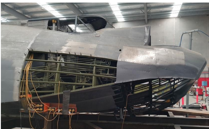
Left image shows the modification being made to the front to install the bow turret. The right image shows where the main wing attaches.
