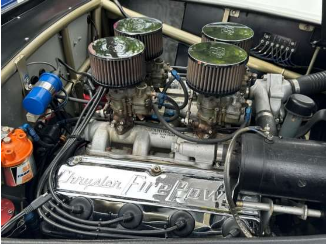
With the special Briggs Cunningham cast intake manifold....
