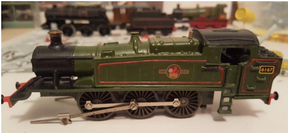
Above pic - This GWR Prairie Tank is getting a Tri-ang chassis taken from a Princess locomotive. The rear set of drive wheels are not in quite the right position but the chassis is from the same era as the kit.
